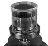
Differentially pumped quartz enclosure for heater elements
